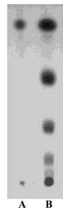
Figure 2. TLC analysis of transglycosylation products: (lane A) daidzin standard; (lane B) transglycosylation products. Spots were visualized by UV detector at 254 nm.
